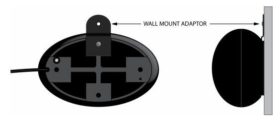
Figure 13. IR Sensor Wall Mount Adaptor
